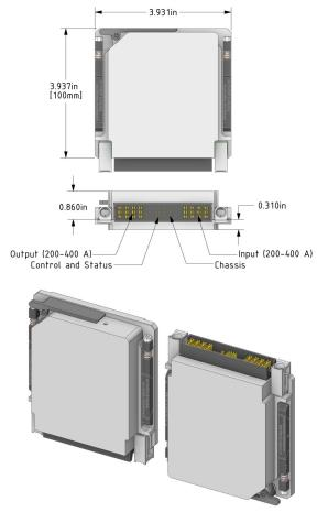
**Figure 8:** High-power sVPX ECB concept for front-end power distribution and controls with lower size and weight over standard 3U.
