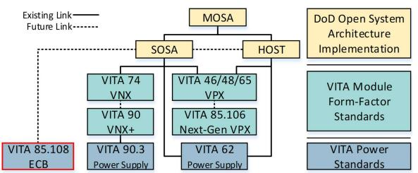
Figure 1: Overview of the landscape of MOSA standards for power, indicating the need for a new power distribution standard to support advanced power controls and PPMx data collection.
