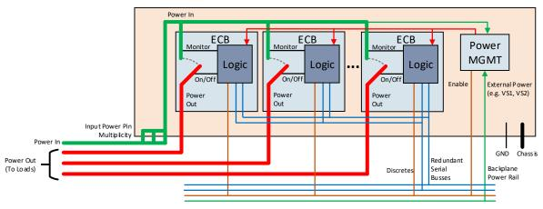
Figure 5: ECB module architecture incorporating the interfaces necessary to meet functional needs of intelligent power management.
